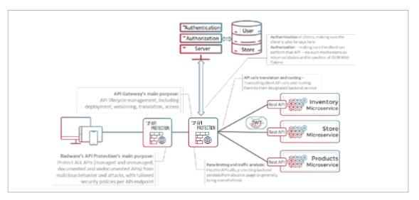
Many API gateways also provide basic API protection capabilities, including authentication and authorization, encryption, rate limiting, transaction logging and rudimentary signature-based security policies.
