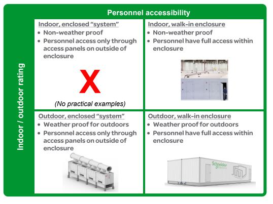
A key driver for choosing an enclosed form factor is the need for the data center subsystems to go outside, or be protected from other elements such as in a hazardous, rugged, or adverse indoor environment. Enclosures that are placed outdoors should have an appropriate level of security to prevent undesirable access (i.e. vandalizing).
